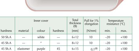
(1) The minimum pulley diameter depends on the overall thickness. (2) Strength in N/mm² at 10% elongation.
